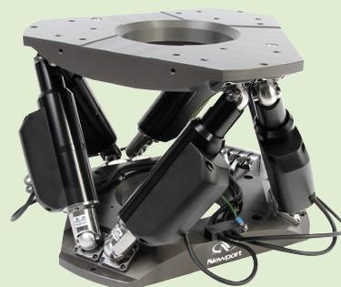
A requirement for many Hexapod motion applications is a virtual pivot point, allowing the user to freely choose the pivot point in space for all rotations. Newport has taken this a step further by providing two pivot points. The two userdefinable coordinate systems provided, called tool (moves with the Hexapod) and work (stationary coordinate system) are programmable and flexible. Imagine a machine tool where one can adjust the
